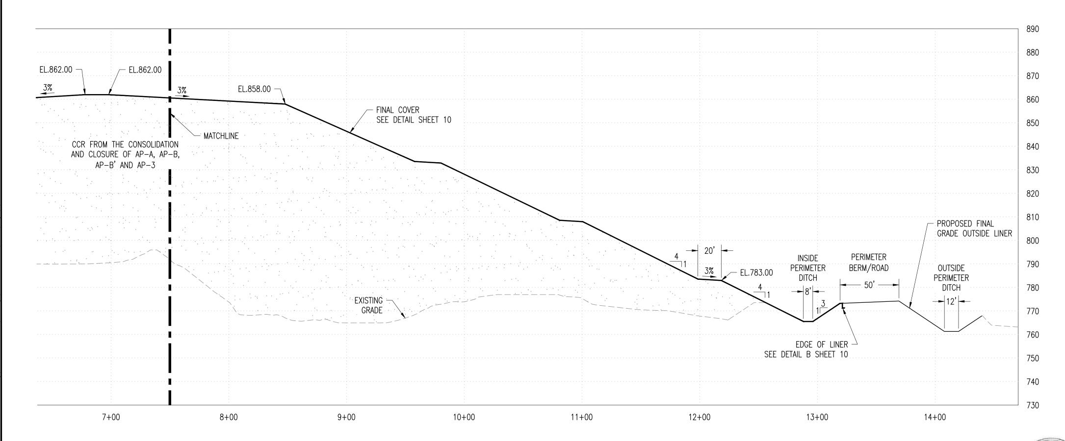
SECTION A SCALE H: 1"= 40', V: 1"=20'
