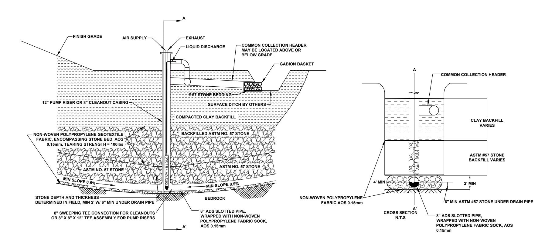
WELL RISER AND COMMON HEADER DETAIL
