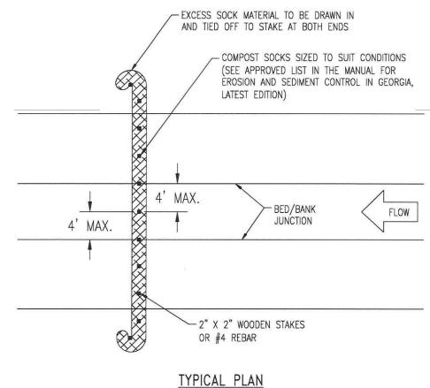
. ALL MATERIAL TO MEET SPECIFICATIONS. 2. PLACE ONE STAKE AT THE CENTER OF THE DITCH/CHANNEL. ALSO PLACE STAKES AT THE BED/BANK JUNCTION AND AT END OF THE DEVICE NOT SPACED MORE THAN 4 FEET APART. 3. CHECK DAMS CAN BE DIRECT SEEDED AT THE TIME OF INSTALLATION.
