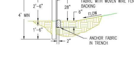
THE SILT FENCE SHALL BE INSPECTED PERIODICALLY AND PROMPTLY REPAIRED OR REPLACED AS REQUIRED. FILTER FABRIC SHALL BE REPLACED WHENEVER IT HAS DETERIORATED TO SUCH AN EXTENT THAT IT REDUCES THE EFFECTIVENESS OF THE
