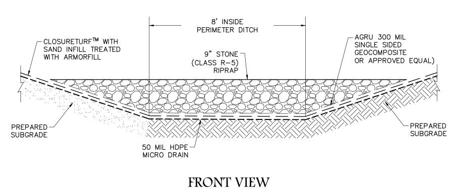
AGRU 300 MIL SINGLE SIDED GEOCOMPOSITE OR APPROVED 9" STONE -(CLASS R-5) RIPRAÉ EQUAL) ┌─ CLOSURETURF<sup>™</sup> WITH SAND INFILL TREATED WITH ARMORFILL PREPARED -50 MIL LLDPE OR-HDPE MICRO DRAIN SUBGRADE SIDE VIEW
