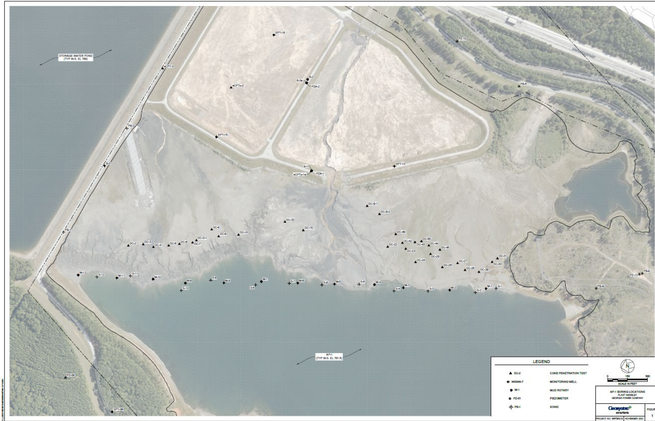
Figure 1. Boring Locations at the Site
