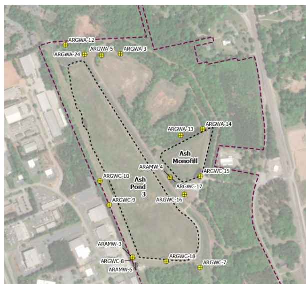
Plant Arkwright Ash Pond 3 Landfill and Monofill
